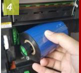
Load take-up spindle, from left to right; make sure collared end of spindle is on the right.
