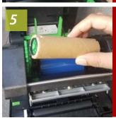
Feed ribbon, back to front, under the print head, taping securely to the take-up spindle. Dull side of ribbon will show.
