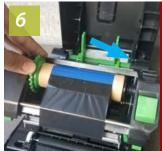
Make sure spindle positions are as shown with larger, collared end on the right.
