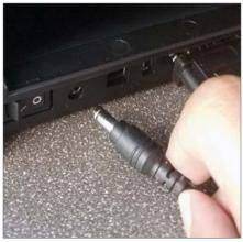
6. Connect power supply cord to printer; connect cord to SURGE PROTECTOR (not supplied, and not a "power strip". This will help protect your printer from power surges and program failures).
