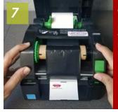
Gently hand-tighten spindles, taking up slack in ribbon.
