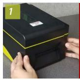
TURN OFF printer; open cover by pressing in on round white tabs on either side of printer.
