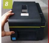
Press ink carriage down, back into printer, close printer cover you're ready to start printing!
