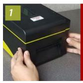
TURN OFF printer; open cover by pressing in on round Green tabs on either side of printer.
