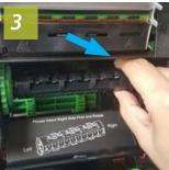
Load rear spindle with ink ribbon, from left to right; make sure collared end of spindle is on the right.
