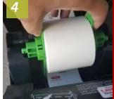
Slide the roll of stickers onto the sticker spindle; lineup spindle guides with spindle slots and place in printer.
