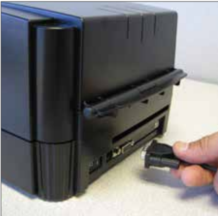
5. Connect the Striker Keypad to the printer
