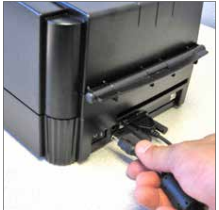
6. Connect power supply cord to printer; connect cord to SURGE PROTECTOR (not supplied, and not a "power strip". This will help protect your printer from power surges and program failures).
